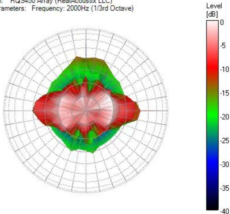
In the Balloon Display view you may select any frequency data set from 25Hz to 20KHz. Some of the lower frequency information will be limited dependent on the size of the specimen. Some of the high frequency information will be less useful due to air absorption. This, however, can be compensated for in the viewer settings. The actual useable frequency response is more along the lines of 250Hz to 10KHz.
