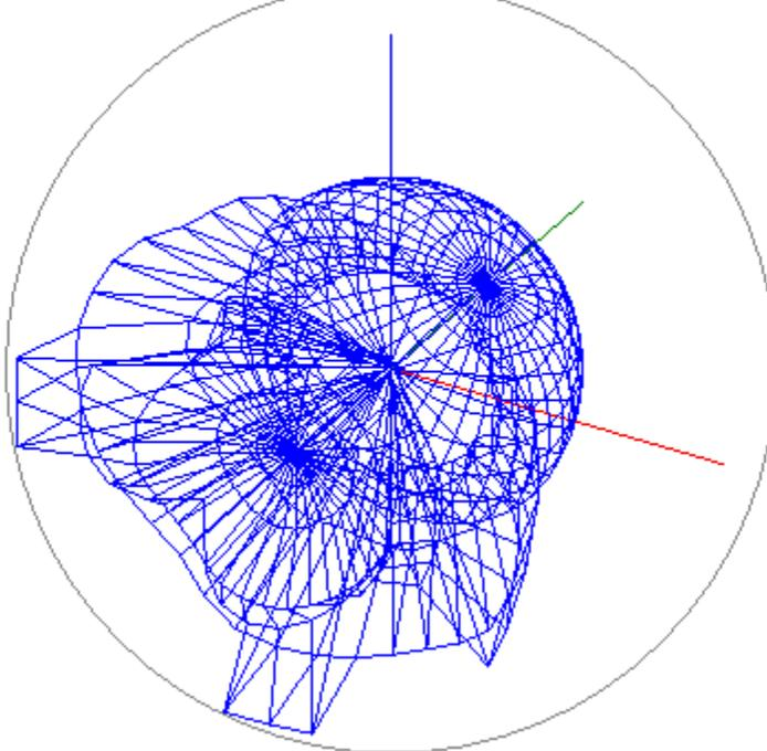
At first glance, this window can confuse those not familiar with phase balloons. Remembering that this is a 1D QRD with a design frequency (LF) of 450Hz, it is natural to assume that we will see mixed phase reflections coming from the DUT.
