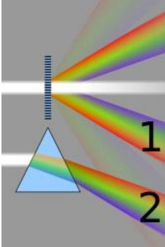
White light is a diffuse light. It is made up of many different colors, or single phase/frequency light waves. This is best represented when a source light is put through a prism (# 2) which acts as a refractor separating the light into its different frequencies or wavelengths.
