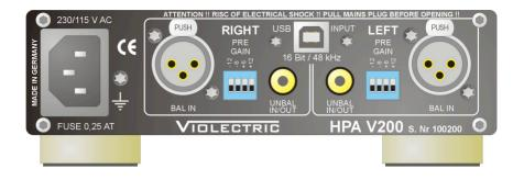
The alignment between amplifier and headphone is provided by the preamp stage, which can boost or attenuate the input signal in four steps of 6dB each. For this purpose, two switching devices are located on the rear panel for left and right channel individually.
