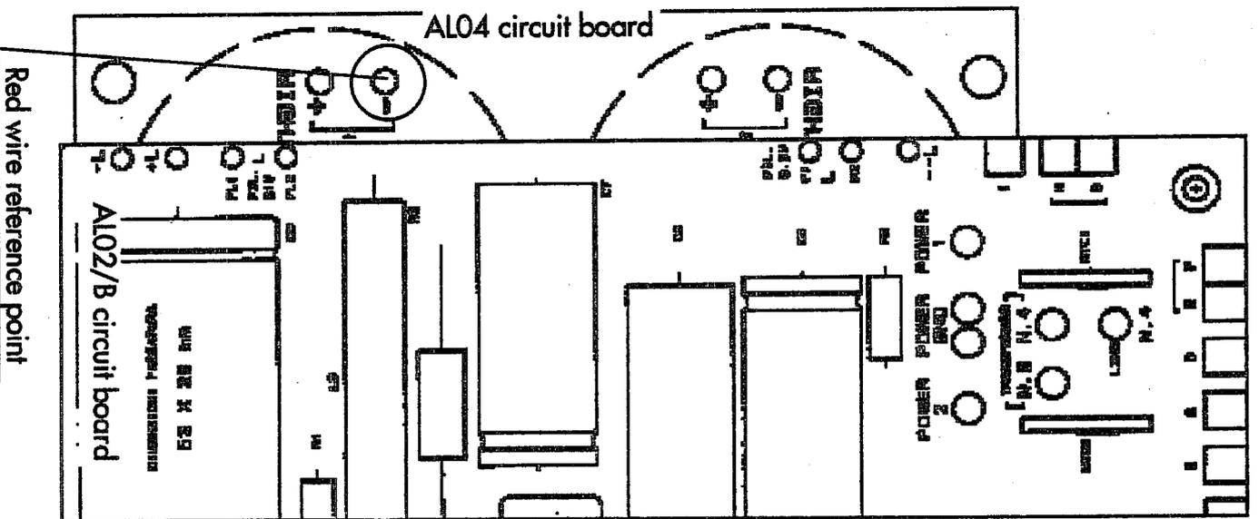
**IMPORTANT:** To have the best performance the amplifier must have the same voltage of the AC line of the country where it is working. To check if the GM 100 has been correctly set, follow the indications of the voltage selection table and check the connection between the transformer wires and the power supply circuit board.
