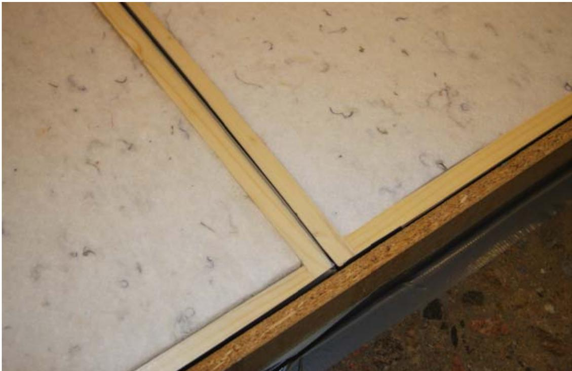
*Picture 2 – A wooden frame was mounted around the test object and sealed with tape against the floor.*
