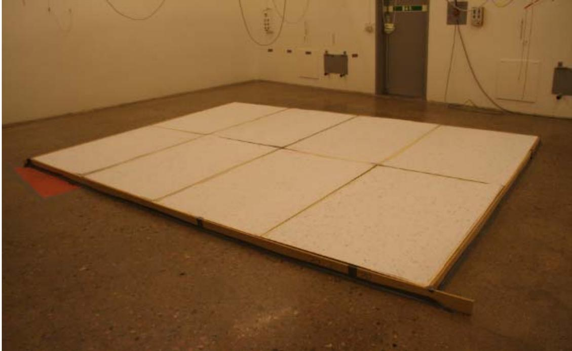
*Picture 1 – Test object mounted in the reverberation room.*
